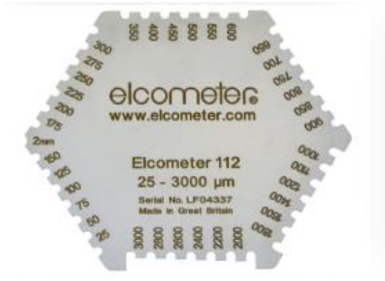
Elcometer 112AL Punched Wet Film Combs (Aluminium)
