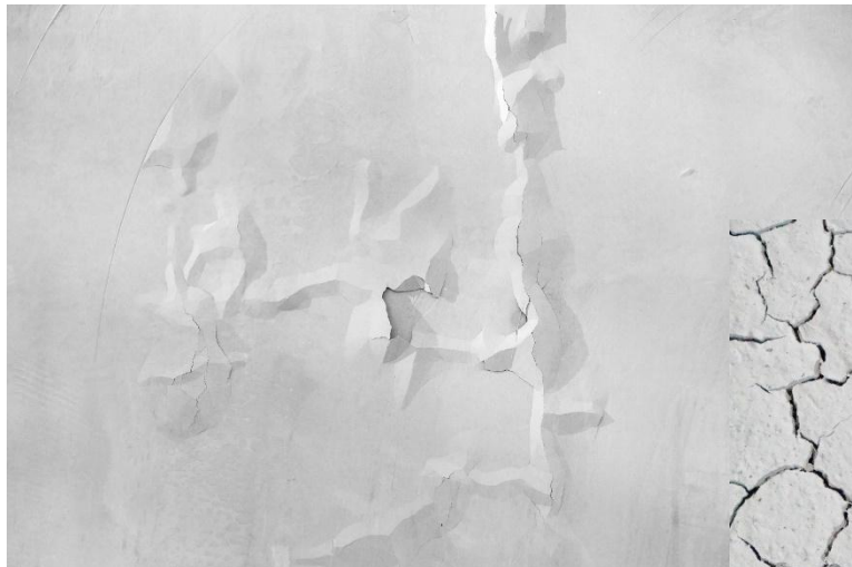
Fig 3. Uncured paint due to too much being applied (Left)
