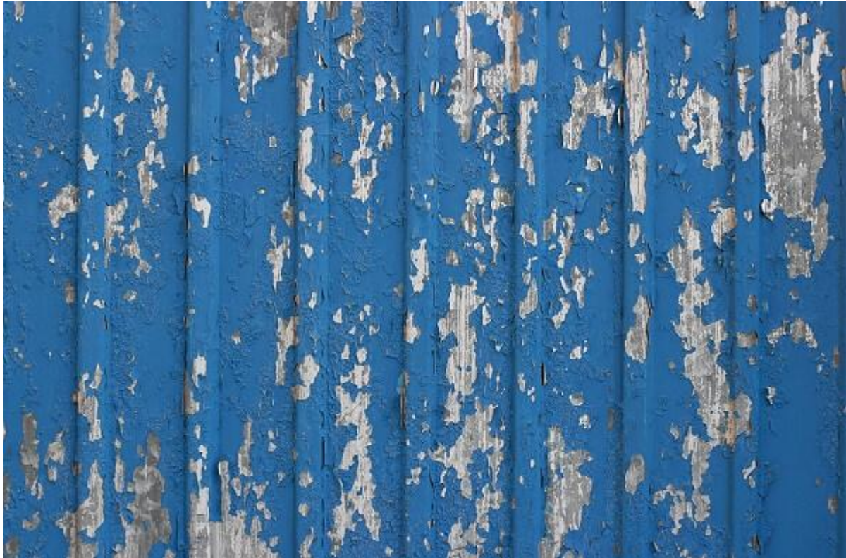
Figure 1. Intercoat adhesion failure (Dmitry Guzhanin / Dreamstime.com).
