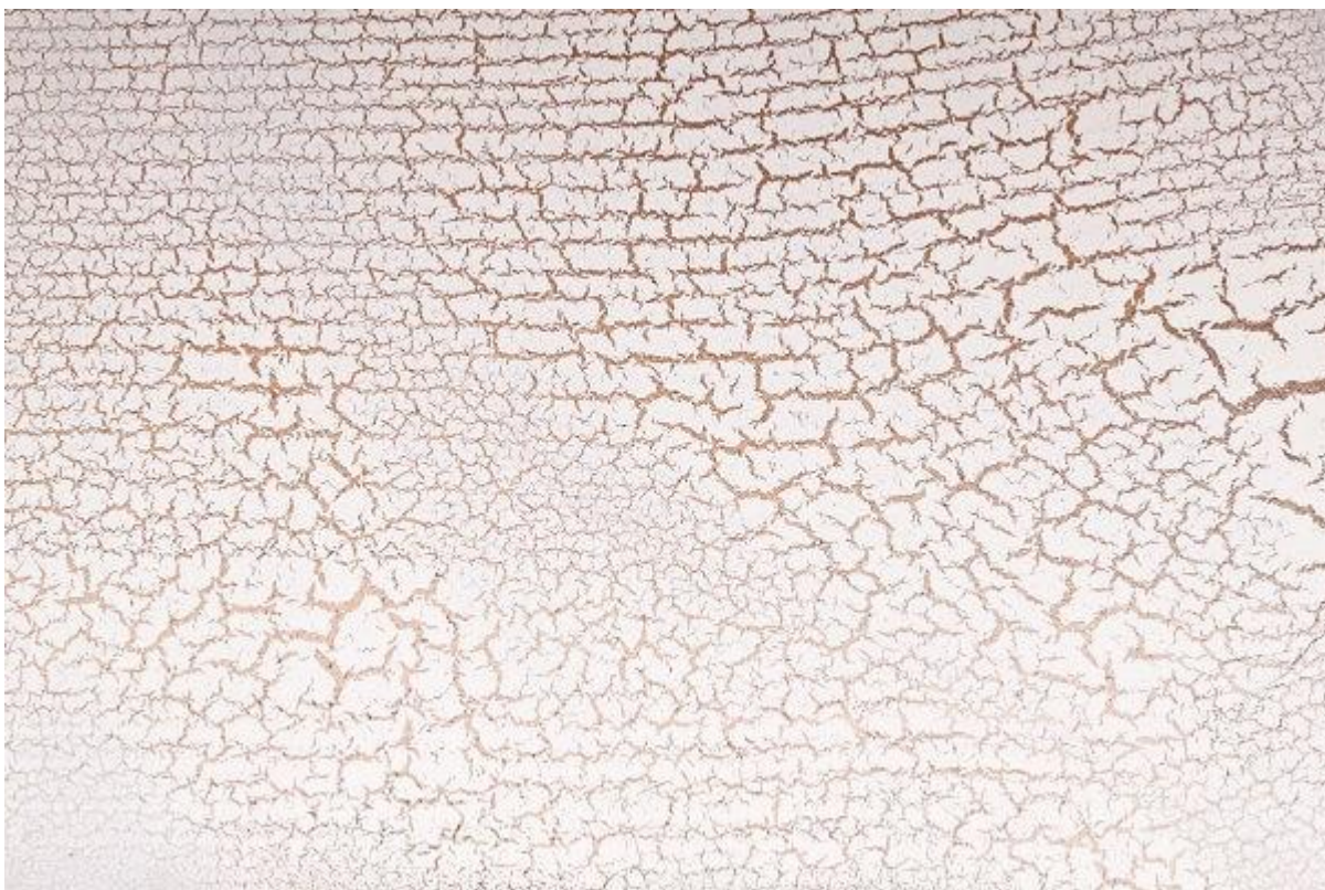
Figure 3. Crazing coating defect (Valentyn75 / Dreamstime.com).
